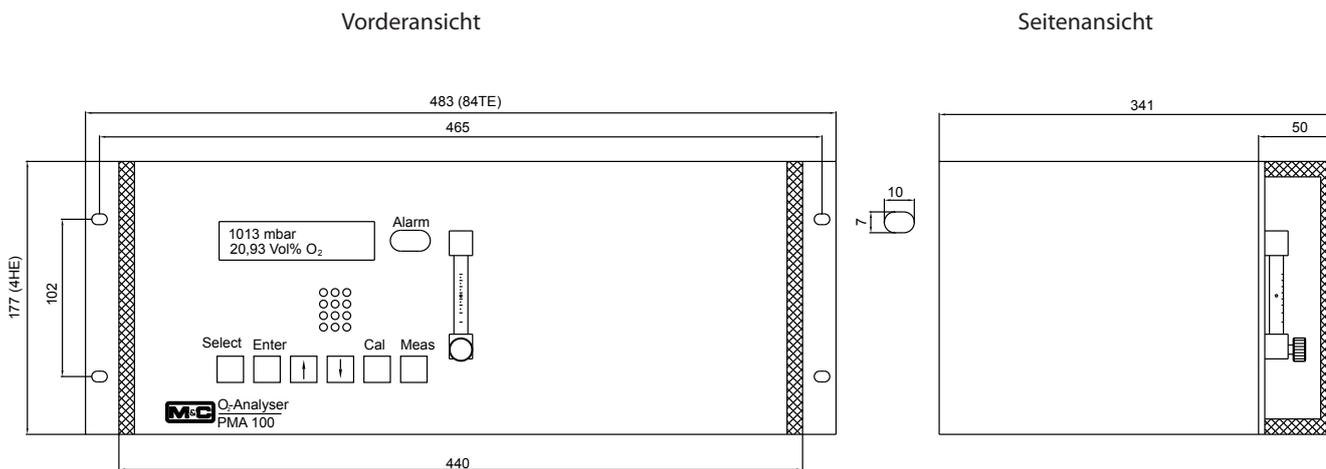
Abmessungen in mm
