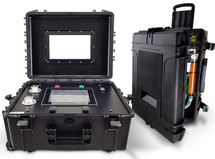
Control and cooler unit of the portable sampling system
