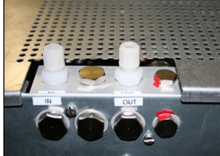
Figure 4 Hose connections for wall mounting or 19"-rack-mounting
