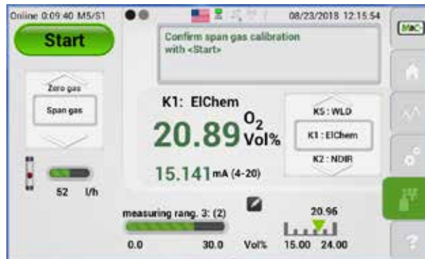
Fig. 76: Manual calibration with span gas
