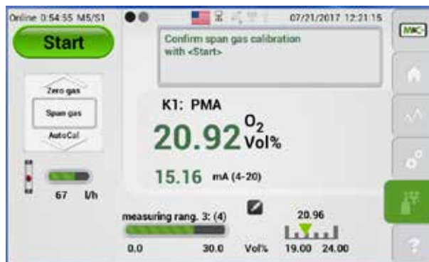
Fig. 68: Manual calibration with span gas
