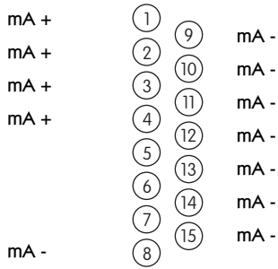
Fig. 8: 15-pole Sub-D socket X3
